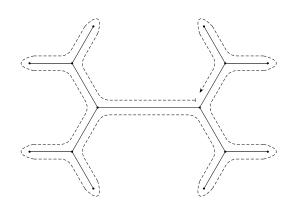
Figure 2.2: Euler traversal of an unrooted tree
