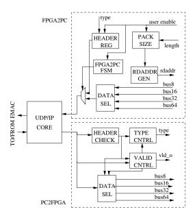
Figure 3. Hardware design of the communication platform.
