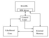
Figure 6. Conceptual design of the complete SW/HW system.
