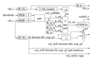
Figure 4. Architecture of the pipelined ancestral vector entry scaling unit.
