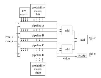
Figure 3. Block diagram of the likelihood core with 4 instances of the PLF pipeline.
