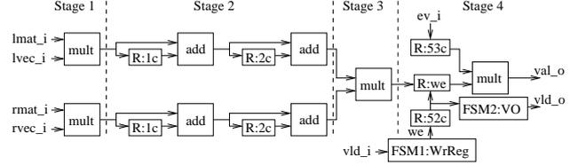
Figure 2. Block diagram of the pipelined PLF architecture for DNA data.
