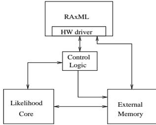
Figure 6. Conceptual design of the complete SW/HW system.
