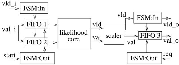
Figure 5. Top-level architecture of the PLF system.
