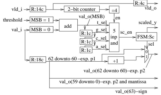
Figure 4. Architecture of the pipelined ancestral vector entry scaling unit.
