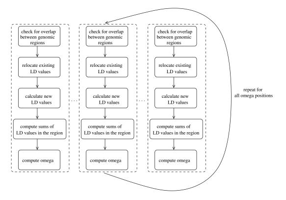
Figure 8.6: Coarse-grain OmegaPlus parallelization.
