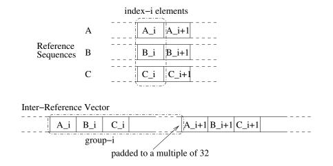
Figure 6.6: Example of the inter-reference memory organization on SIMD and SIMT platforms. All index-i elements are grouped together in group i. Groups are padded to a multiple of 32 for performance reasons.
