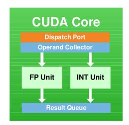
Figure 3.8: Schematic representation of a CUDA core. (Source: [144])
