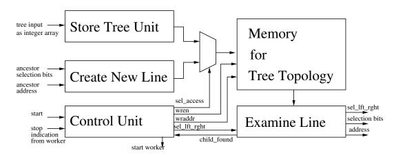
Figure 5.7: Architecture of the Target Pair Unit (TPU).
