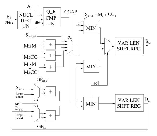
Figure 6.2: The scoring cell (SC) architecture.
