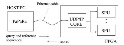
Figure 6.4: The FPGA-based acceleration system.
