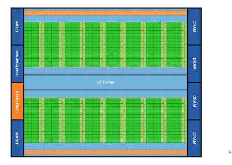
Figure 3.10: Overview of the Fermi architecture. Fermi's 16 SMs are positioned around a common L2 cache. Each SM is a vertical rectangular strip that contains an orange portion (scheduler and dispatch), a green portion (execution units), and light blue portions (register file and L1 cache). (Source: [144])
