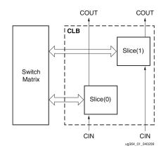
Figure 3.2: Arrangement of slices within the CLB. (Source: [208])
