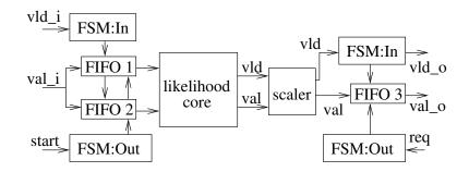
Figure 5.20: Top-level architecture of the PLF system.
