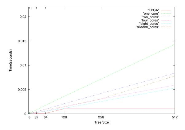
Figure 5.5: FPGA and multi-core execution times for full tree traversals using Felsenstein's pruning algorithm for trees with 4, 8, 16, 32, 64, 128, 256, and 512 taxa.
