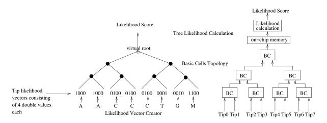
Figure 5.3: Example for the computation of the likelihood score on a single alignment column for an 8-taxon tree using the Likelihood Vector Creator, Basic Cell, and Tree Likelihood Calculation units.
