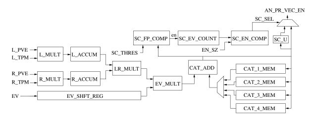
Figure 5.13: Block diagram of the NV\_PRU processing unit.
