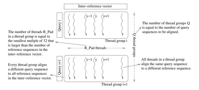
Figure 6.7: Example of the inter-task parallelization strategy. Thread y of group i aligns QS i to RS y. The number of threads in a thread group depends on the number of RS in the interreference vector. The number of thread groups depends on the number of QS. Every thread group aligns a different QS to all RS, and all threads in a thread group align the same QS to all RS.
