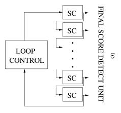
Figure 6.3: Loop control mechanism for accommodating query sequence lengths that are larger than the number of available SCs.
