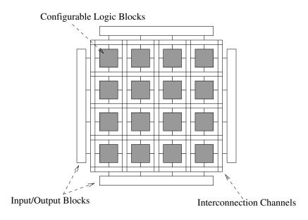
Figure 3.1: Simplified FPGA floorplan.
