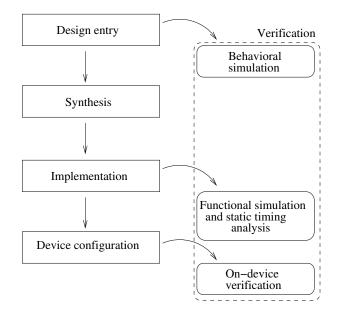
Figure 3.5: Traditional FPGA design flow.
