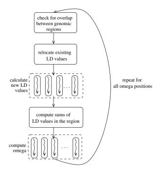
Figure 8.5: Fine-grain OmegaPlus parallelization.
